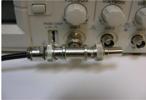
Figure 4: BNC T-Adapter on the oscilloscope with coaxial transmission line connected on the left and BNC 50 \Omega resistor connected on the right to terminate the line.
