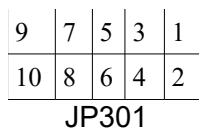
Figure 12: HW_Trig/Reset Header Pin-Out (SP57 and SP58). Top-down view.
