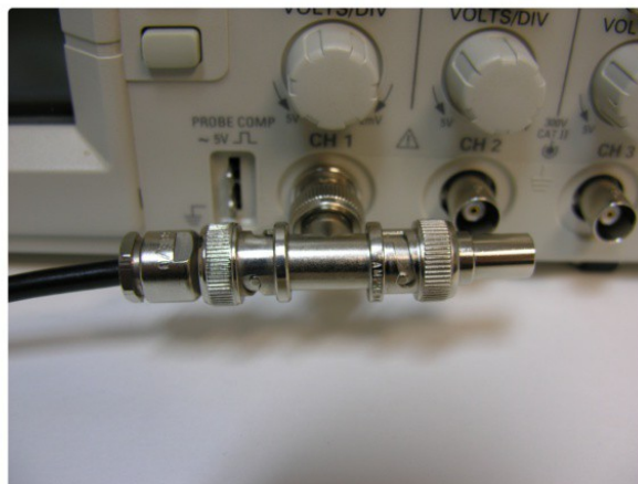
Figure 11: BNC T-Adapter on the oscilloscope with coaxial transmission line connected on the left and BNC 50 Ohm resistor connected on the right, to terminate the line.
