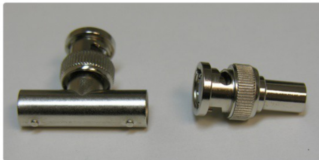
Figure 10: Left: BNC T-Adapter and Right: BNC 50 Ohm resistor.
